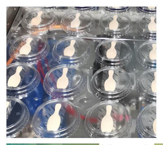
Spoon inserted directly during production. The spoon is in a bag, totally untouched by human hands. Pack Plast recycles almost all its plastic materials. Leftover foil is collected, pressed and returned to the supplier.
